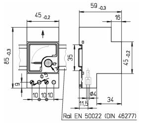
Picture 6: Dimensional drawing BQ0507 (all dimensions are in mm)
