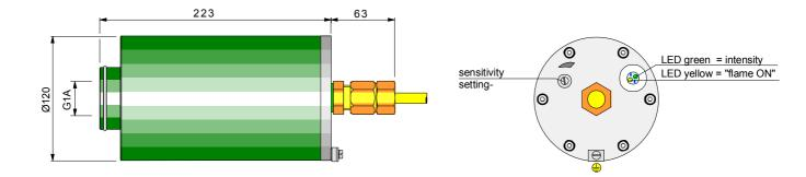
Class: EEx d IIC T 6 for PTB 87/1095
